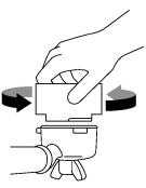
• Wipe excess coffee from the rim of the filter basket to ensure a proper seal is achieved in the group head.
